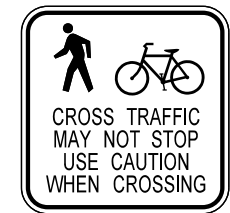
W11-501 (12" x 12") PEDESTRIAN SYMBOL HEIGHT - 4" (IN) BICYCLE SYMBOL HEIGHT - 3" (IN) LETTERS - 1" C LEGEND - BLACK BACKGROUND - YELLOW
