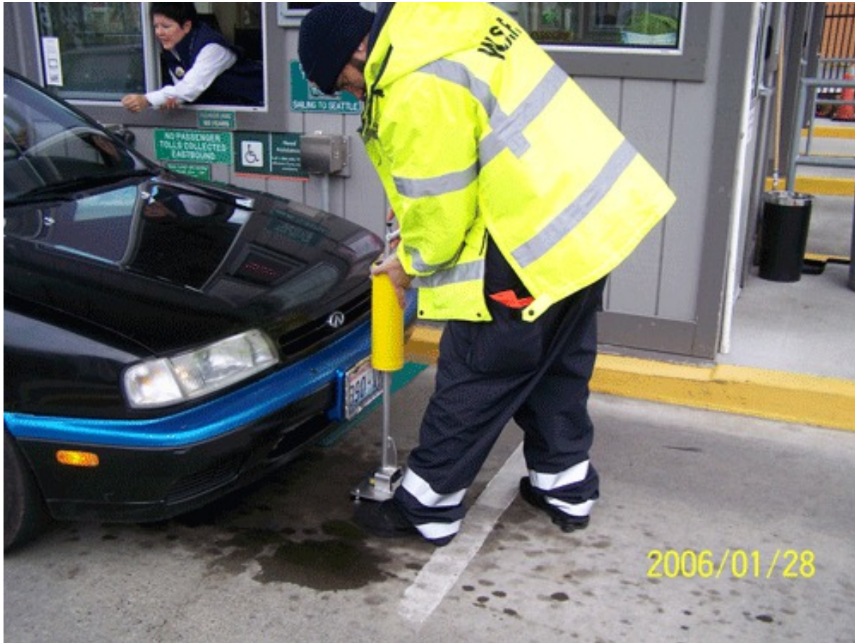
A state ferry worker measures vehicle length using WSF's new laser-equipped measuring device. — image credit: Courtesy of Washington State Ferries
