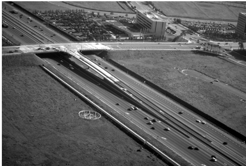
Drop ramp photograph from FHWA/PB HOV Interactive 1.0 High Occupancy Vehicle Data Base from the U.S., Canada, and Europe
