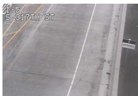
HOV Entrance sign located on the right side at the beginning of each on-ramp.
