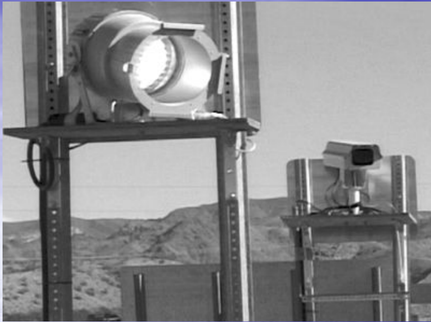
Arizona Route 68 License Plate reader used to measure travel time
