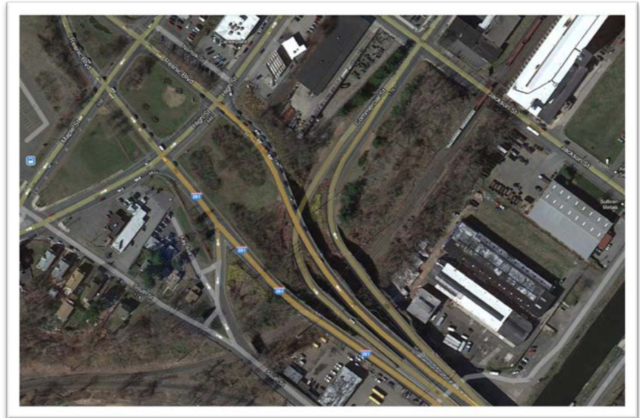
Figure 2-11: Example of an Interstate Spur Terminating at a City Street in Holyoke, MA
