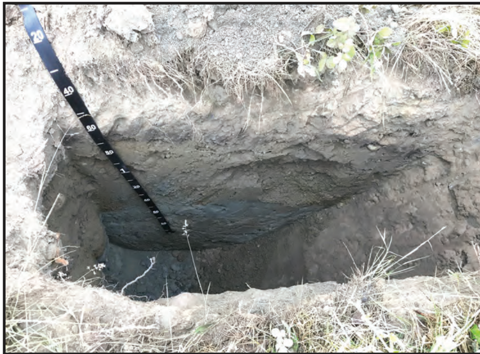
Exhibit 6-62. Pit 20 south wall profile. The pit was excavated to 240 cm below surface, exposing a profile consisting entirely of fill. Pockets of the fill have a bluish-gray color, indicating an origin from low-lying, wetland areas where soils would be saturated. The scale consists of 10-cm long increments.
