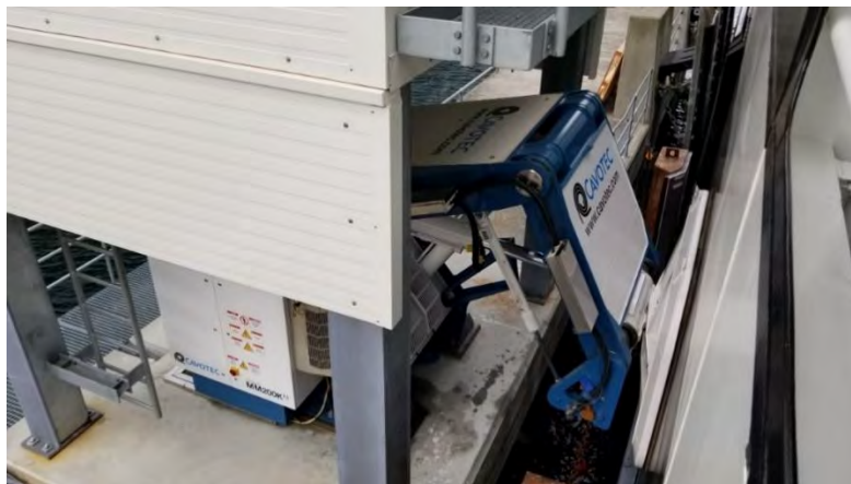
Figure 11: Cavotec MoorMaster Automated Vacuum Mooring System
