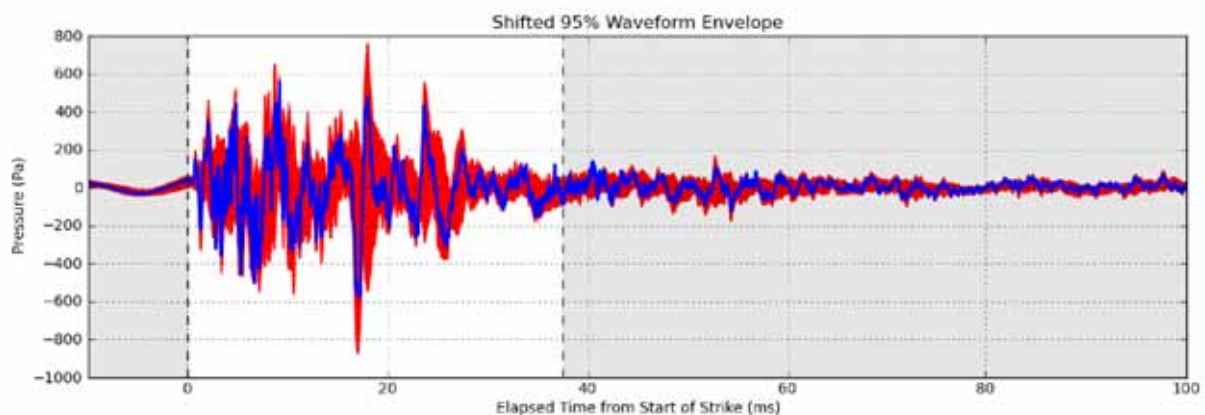
FIGURE 3-5. 95 PERCENT WAVEFORM ENVELOPE (RED) WITH SINGLE COMPONENT STRIKE WAVEFORM (BLUE). 90 PERCENT OF THE ENERGY OF THE STRIKE LIES BETWEEN THE SHADED REGIONS.
