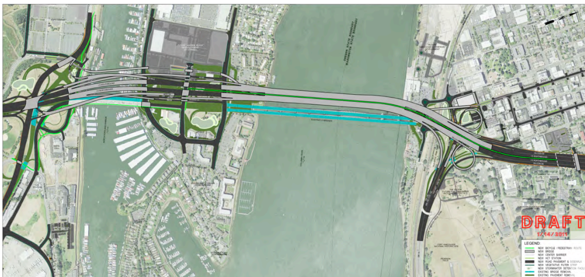
Figure 39 – Tangent Downstream Alignment
