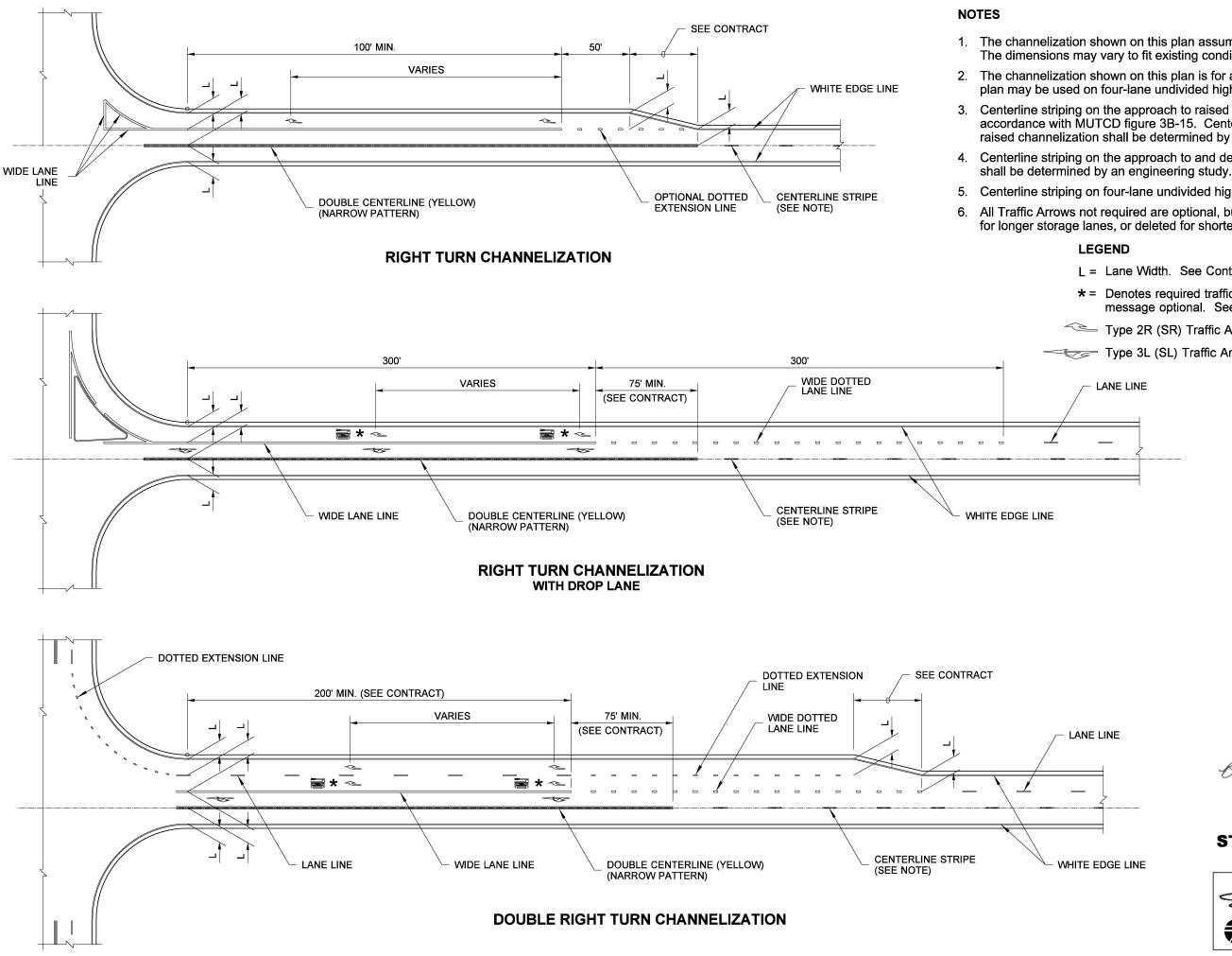
1. The channelization shown on this plan assumes optimal roadway geometric design. The dimensions may vary to fit existing conditions. See Contract.
