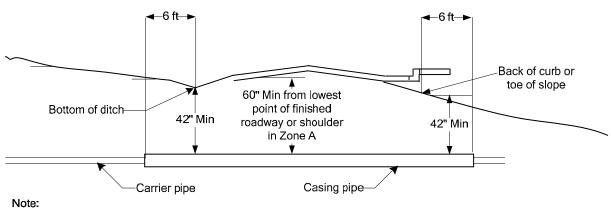
Casing pipes shall extend a minimum of 6 feet beyond the toe of fill slopes, or bottom of ditch line, or outside curb.
