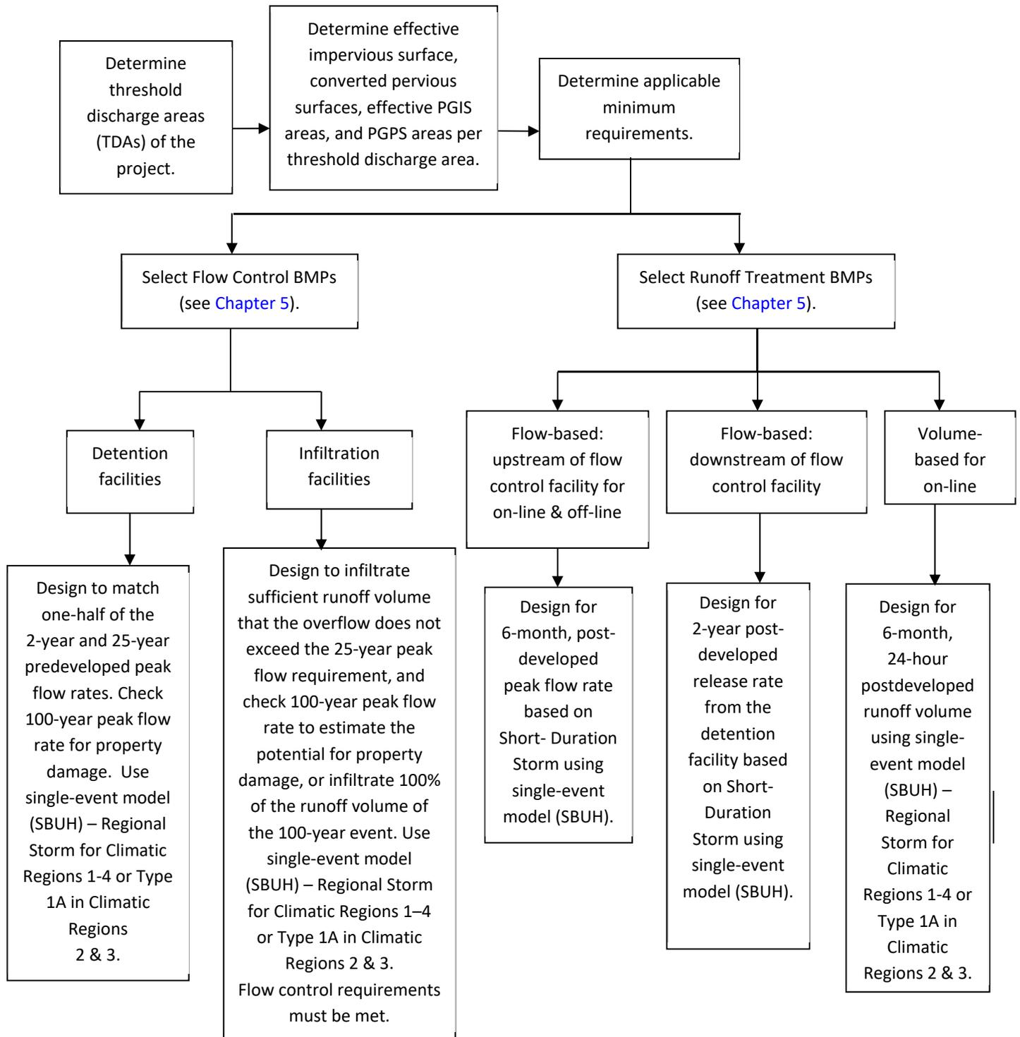
Figure 4-5 Hydrologic analysis flowchart for eastern Washington.
