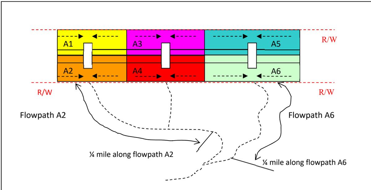
Figure 4-2 Threshold discharge areas (plan view)
