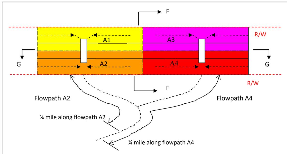
**Figure 4-1** Threshold discharge areas (plan view)
