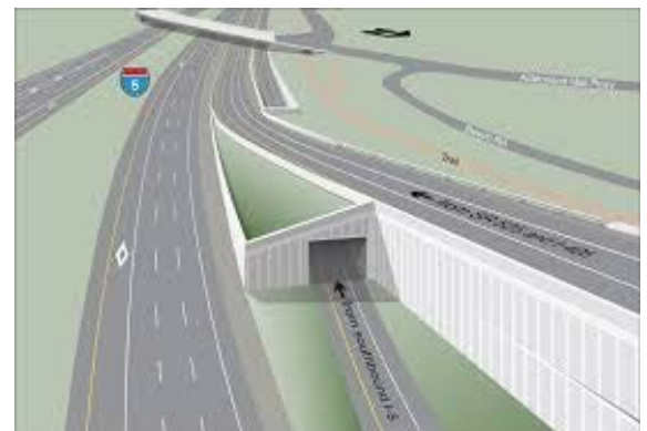
Braided ramp and local street overpass
