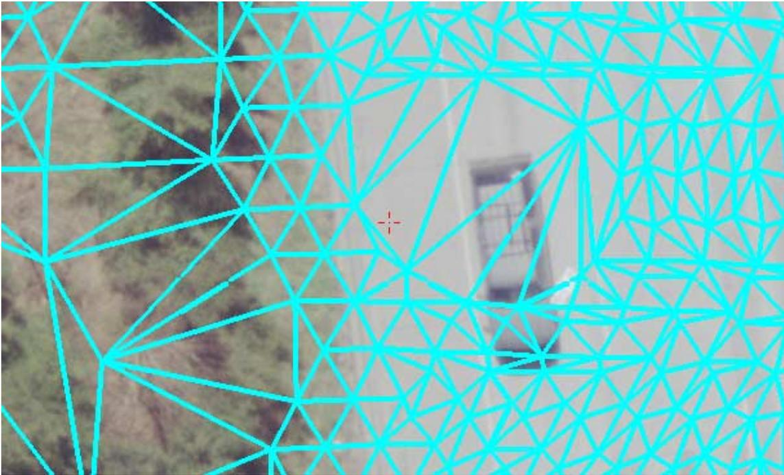
*PSLC IDAR digital Terrain Model (DTM) draped over WSDOT 1:3000 photo scale aerial photography in a 3.D. Photogrammetric Soft Copy System.*
