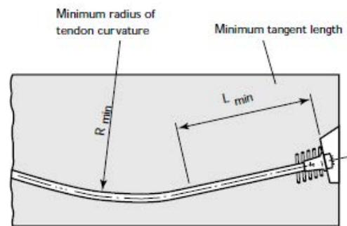
Figure 1: Tangent Length and Tendon Radii
