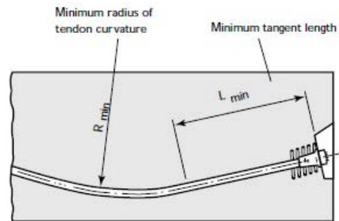
Figure 5.8.1-4A: Tangent Length and Tendon Radii
