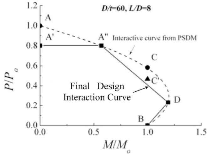
Fig. 4. Construction of the Stability-Based Interaction Curve for CFT and RCFT
