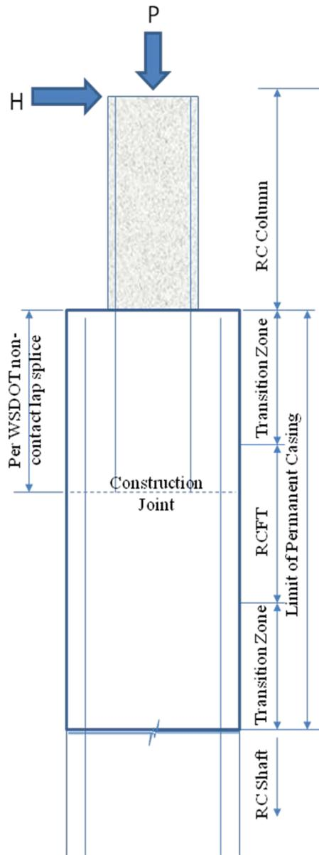
Figure 8. RC to RCFT connection
