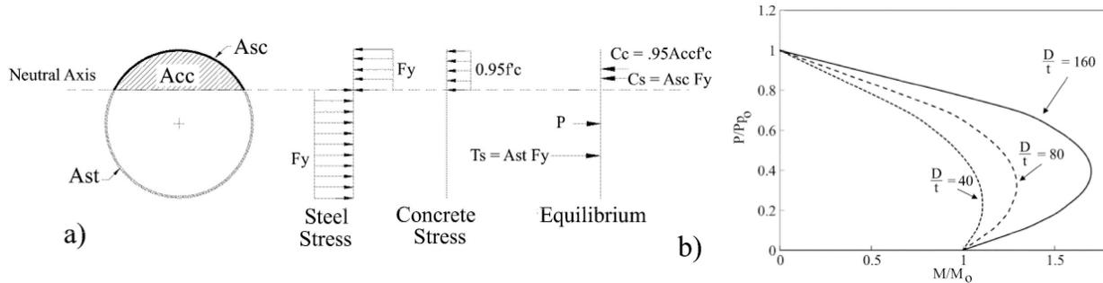
Fig 1. Strength determination for CFT; a) Plastic stress distribution method, b) Material-based interaction curves (no buckling)
