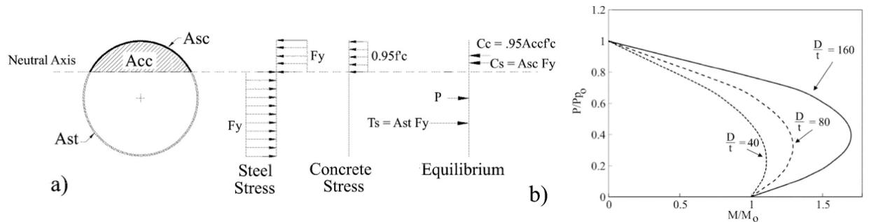
Fig 7.10.1 Strength determination for CFT; a) Plastic stress distribution method, b) Material-based interaction curves (no buckling)
