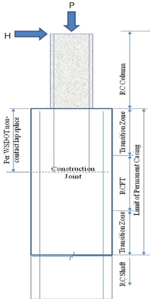
Figure 7.10.8. RC to RCFT connection
