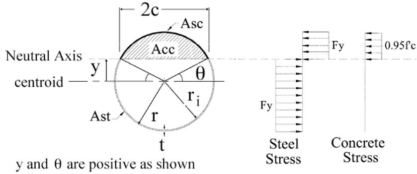
Fig. 7.10.2 Geometry used for closed form derivation of CFT stress distribution prediction
