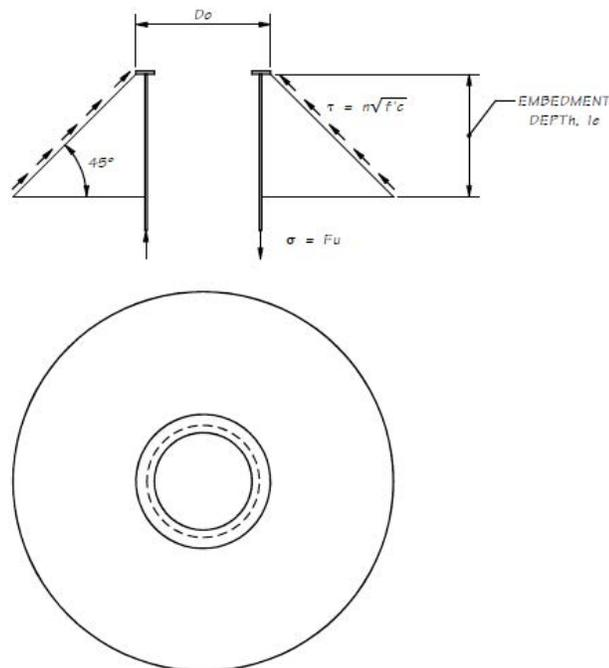
Fig. 7.10.5. Cone pullout requirements for the full strength pile cap connection
