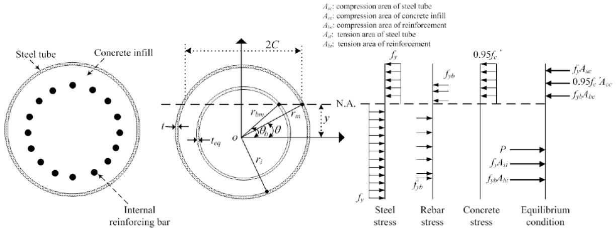
Fig. 3. Geometry for derivation of plastic stress distribution method for RCFT
