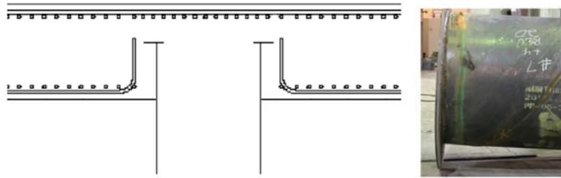
Fig. 7.10. 7. Detailing of longitudinal reinforcement adjacent to the tube
