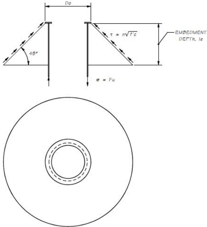
Fig. 5. Cone pullout requirements for the full strength pile cap connection
