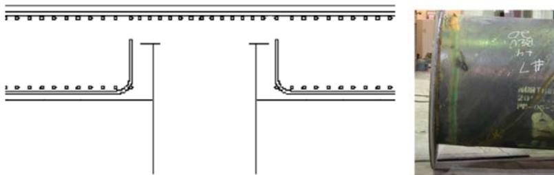
Fig. 7. Detailing of longitudinal reinforcement adjacent to the tube
