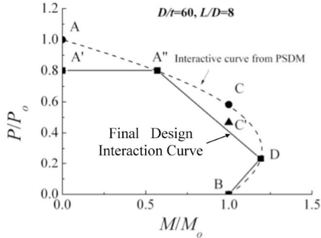
Fig. 7.10.4. Construction of the Stability-Based Interaction Curve for CFT and RCFT
