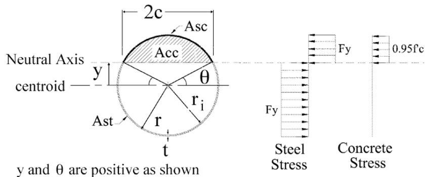
Fig. 2. Geometry used for closed form derivation of CFT stress distribution prediction
