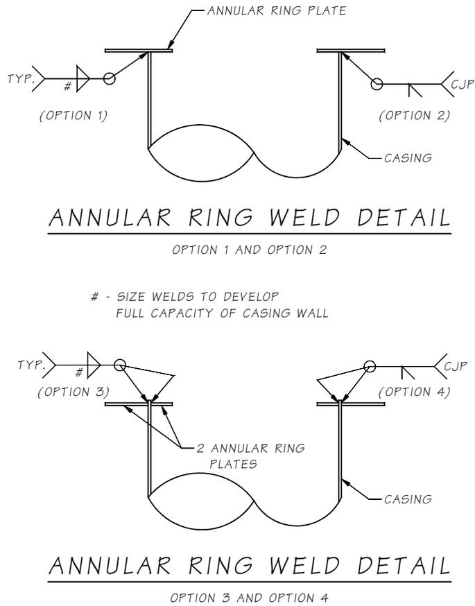
Figure 6. CFT Weld Detail
