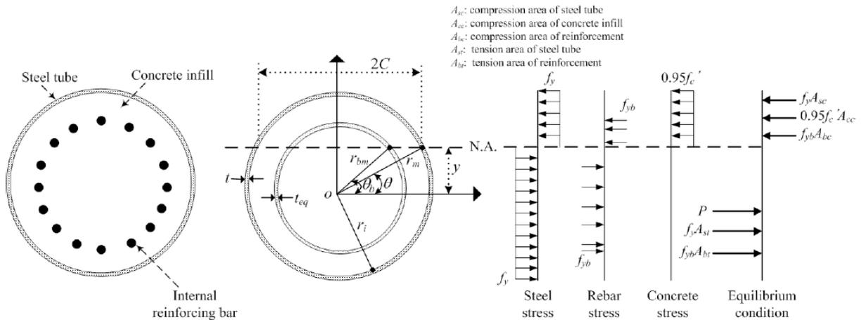
Fig. 7.10.3. Geometry for derivation of plastic stress distribution method for RCFT
