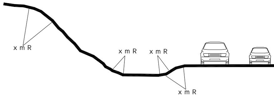
"x m R" represents the meter radius needed to meet the design intent and blend into surrounding landforms.
